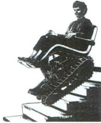
FIGURE 5. Wheelchair adapted to up and down stairs.
